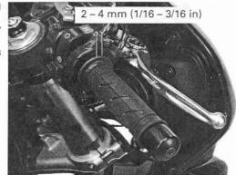
Throttle grip free play can be adjusted at either end of the throttle cable.
