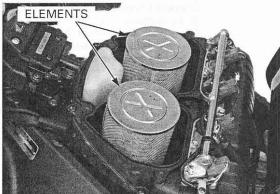
Install the air cleaner elements while aligning their bosses with the grooves in the air cleaner housing.
