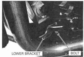
Install and tighten the radiator lower mounting bolt.
