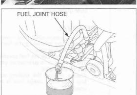
After inspection, install a new O-ring into the groove of the fuel joint hose.
