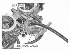
Release the thermal valve shaft joint piece from the thermal valve link arm, then remove the thermal valve assembly.
