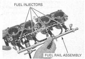
Tighten the fuel rail mounting bolts to the specified torque.
