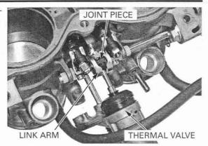
Tighten the thermal valve mounting screws to the specified torque.
