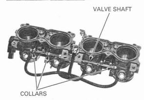
during disassembly so they can be placed back in their original locations.
