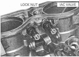
Check the IAC valve for scratches, scoring or other damage, replace it if necessary.
