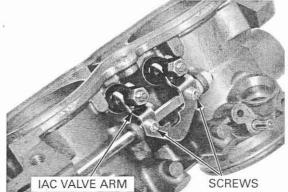
Remove the IAC valve shaft and three collars.
