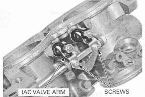
Turn the IAC valve screw until it seats lightly, then back it out as noted during removal.
