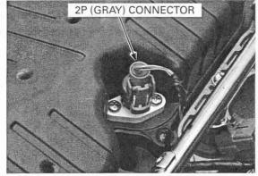
Remove the screws and IAT sensor from the air cleaner housing.
