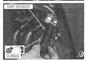
Connect the CMP sensor 2P (Black) connector. Install the removed parts in the reverse order of removal.
