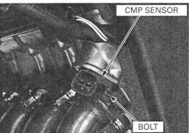
Apply oil to a new O-ring and install it onto the camshaft position sensor groove.
