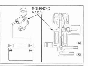
Check the resistance between the terminals of the bypass control solenoid valve.
