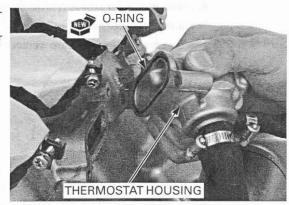
Install and tighten the thermostat housing mounting bolts securely.
