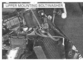
Be careful not to Move the radiator assembly to the right and release damage the radiator the radiator upper grommet from the bracket boss, fins. then remove the radiator assembly.
