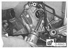
Align the water pump shaft groove with the oil pump shaft end by turning the water pump impeller.
