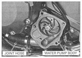
Install a new O-ring into the groove in the water pump cover.
