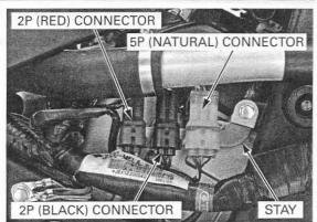
Remove the rear brake light switch wire from the clamps on the right crankcase cover.
