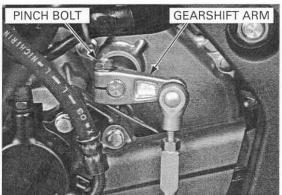
Remove the bolt, washer, wave washer and gear shift pedal assembly.
