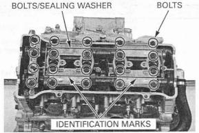
First gradually tighten the four bolts (No.5 – No.6 – No.7 – No.8) in the numerical order cast on the camshaft holders.
