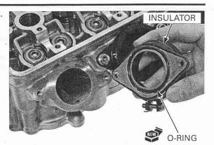
Install and tighten the insulator mounting socket bolts to the specified torque.
