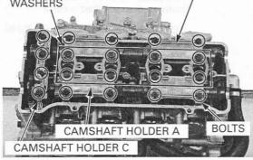
First gradually tighten the four bolts (No.5 - No.6 -No.7 - No.8) in the numerical order cast on the camshaft holders.
