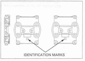
Apply engine oil to the threads and seating surfaces of the camshaft holder bolts.
