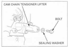
Turn the tensioner shaft fully in (clockwise) and secure it using the special tool to prevent damaging the cam chain.
