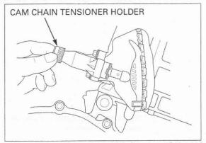
Remove the bolts, sealing washers, cam chain tensioner lifter and gasket.
