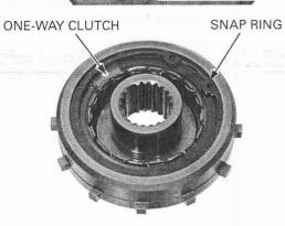
Check the starter clutch outer inner surface and oneway clutch for abnormal wear or damage and replace them if necessary.
