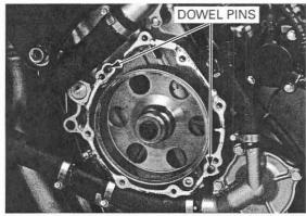
The alternator cover (stator) is magnetically attracted to the flywheel, be careful during installation.
