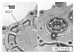
Apply a locking agent to the mainshaft bearing set plate bolt threads and shift drum bearing set plate bolt threads.
