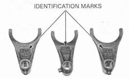
Install the shift forks into the shift drum guide groove with the identification marks facing up.
