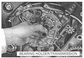
Install and tighten the bearing holder mounting bolts to the specified torque.
