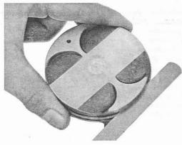
the cylinder with the top of the piston to be sure they are squarely in the cylinder.
