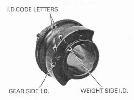
Reference the balancer weight I.D. code letters to determine the replacement bearing color. Refer to the selection table below for bearing selec-
