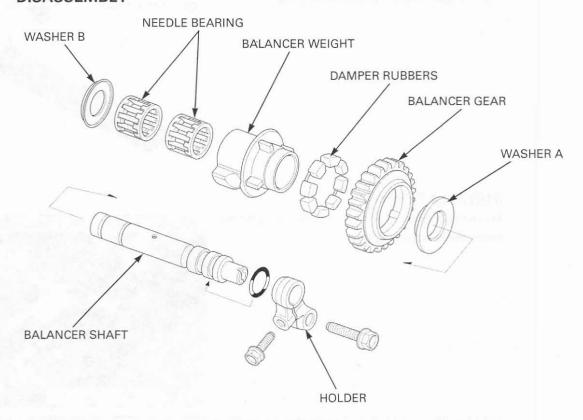
Install the damper rubbers into the balancer gear.
