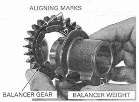
Apply oil to the needle bearing, install them into the balancer weight.
