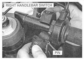
Tighten the screws to the specified torque.
