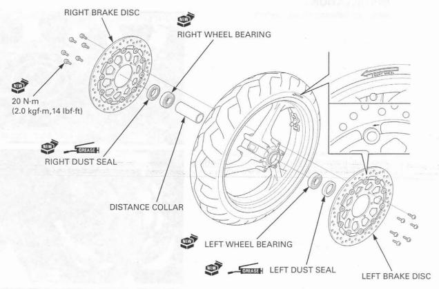
removed, the bear- wheel bearing using the same tools. ings must be replaced with new ones.
