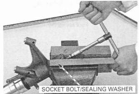
Remove the fork damper assembly from the fork slider.
