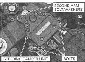
Disconnect the 2P (Black) connector from the steering damper unit.
