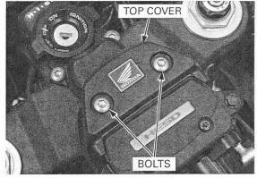
Remove the bolts and steering linkage cover.
