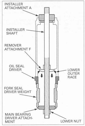
Install a new upper bearing outer race with the special tools as shown.
