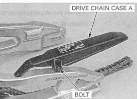
Install the drive chain slider mounting bolt (front). Install the collars and new drive chain slider mounting bolts (rear).
