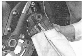
Remove the pad pins, brake pads and pad spring.
