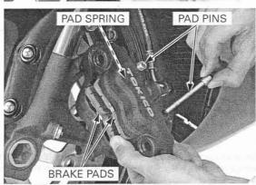
Clean the inside of the caliper especially around the caliper pistons.
