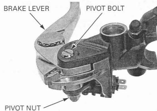
Remove the screw and brake light switch.
