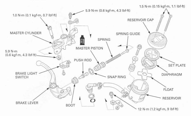
· Keep the piston, cups, spring, snap ring and boot as a set; do not substitute individual parts.
