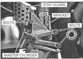
Remove and discard the brake pedal joint cotter pin. Remove the nut, washers, joint bolt and rear master cylinder.
