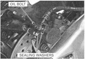
Remove the caliper mounting bolt and the brake pads (page 16-13).
