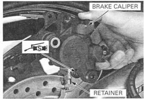
Install the brake hose eyelet joint to the caliper body with new sealing washers and oil bolt.
