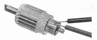
Check for continuity between each commutator bar and the armature shaft.
