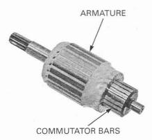
Check for continuity between pairs of commutator
