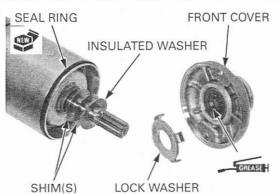
Make sure the index lines are aligned. Install the new O-rings onto the motor case bolts. Install and tighten the case bolts securely.
