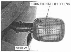
While pushing in, turn the bulb counterclockwise to remove it and replace with new one.
