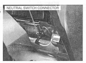
Shift the transmission into neutral and check for continuity between the Light green wire and body ground.
