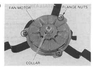
Install the cooling fan onto the fan motor shaft by aligning the flat surfaces.
