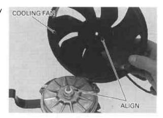
Apply a locking agent to the cooling fan nut threads. Install and tighten the nut to the specified torque.
