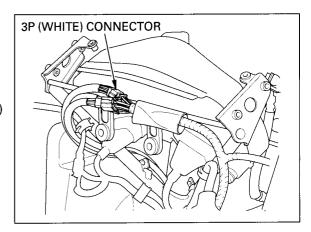
Check for continuity between the wire terminals of the ignition switch connector in each switch position.
